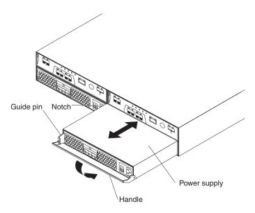
Figure 48. Replacing a power-supply unit
